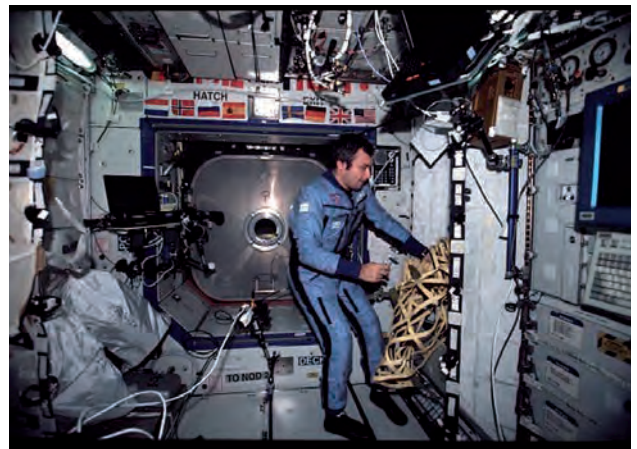
Fig. 9. Vladimir Dezhurov performing test of ARIS ICE-3 experiment stabilization rack by hitting it with a hammer (source: NASA)
