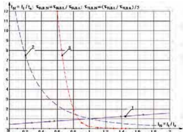
Fig. 2. Dependencies of normalized values of quantities: 1 – temperature of p-n junction ( t_n ) and 2 – ADG of SLS ( \tau_{SLS} ) from normalized values of the current, 3 – AFG of TLS ( \tau_{SLS} ) from normalized values of voltage U_N
