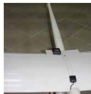
Fig. 12. GPS antenna and GPS tracker mounted on upper skin of center-wing
