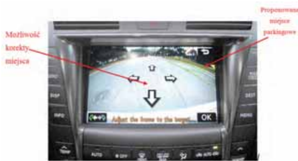
Rys. 1. Toyota – Intelligent Parking Assist System (IPAS) Fig. 1. Toyota – Intelligent Parking Assist System (IPAS)
