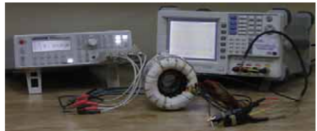
Fig. 4. Laboratory stand to measure electrical parameters of bearingless motor stators
