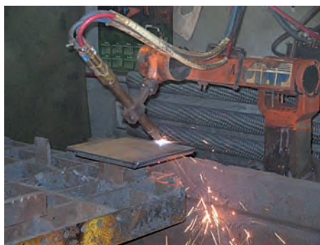
Fig. 2. Industrial robotic system for metal sheets bevelling [www.piap.pl]
