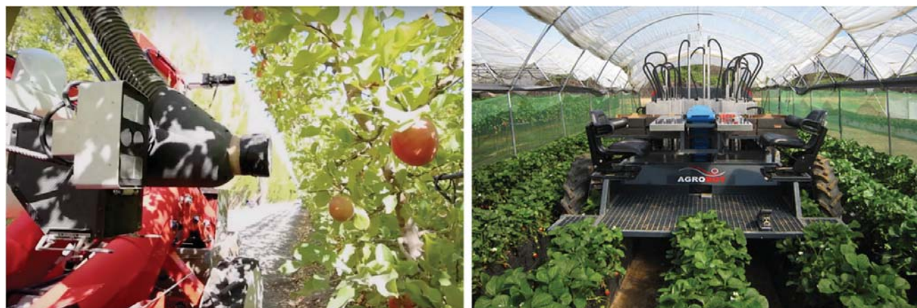
Fig. 3. a) The Apple-picking robot by the Abundant Robotics [4], b) SW6010 robot to harvest strawberries [3] Rys. 3. a) Robot do zbierania jabłek firmy Abundant Robotics [4], b) Robot SW6010 do zbioru truskawek [3]
