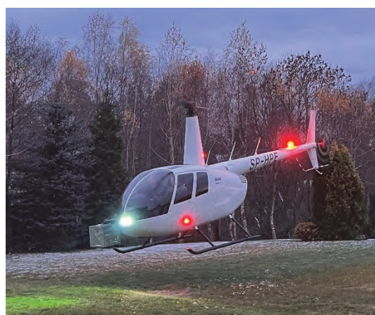
Fig. 1. Measurement subsystem: Robinson R44 helicopter with mounted imaging Fourier infrared spectroradiometer
