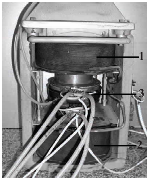
Fig. 1. Device for thermal annealing of ring-shaped cores in transversal magnetic field: 1, 2 – magnet polepieces, 3 – furnace with ring-shaped core
