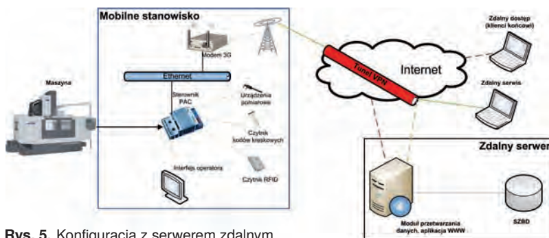
Fig. 5. Configuration with remote server
