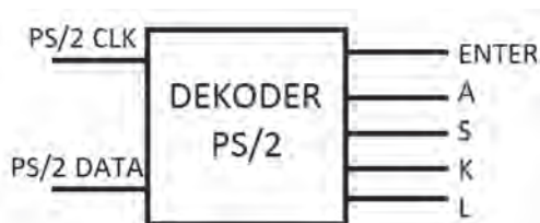
Rys. 4. Schemat zaimplementowanego dekodera PS/2 Fig. 4. Block diagram of implemented PS/2 decoder
