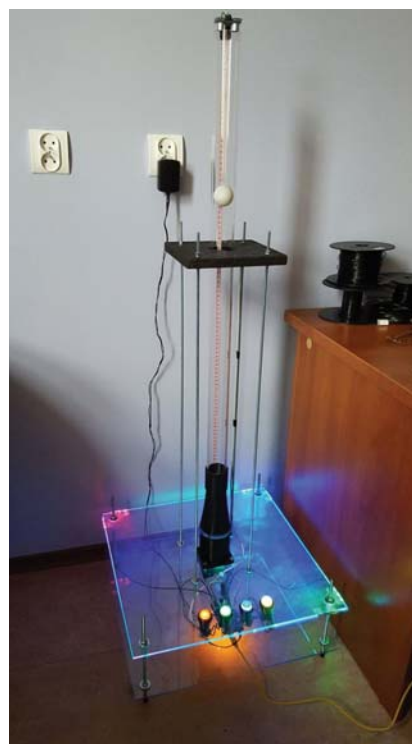
Fig. 2. An assembled air levitation system. The controller senses the position of the object with ultrasonic sensor and drives the current in the fan to maintain levitation
