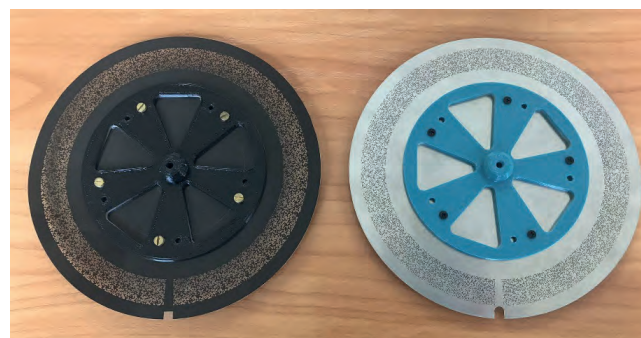
Fig. 7. Two types of SLMs – from the left made of photographic film and on the right made of aluminum
