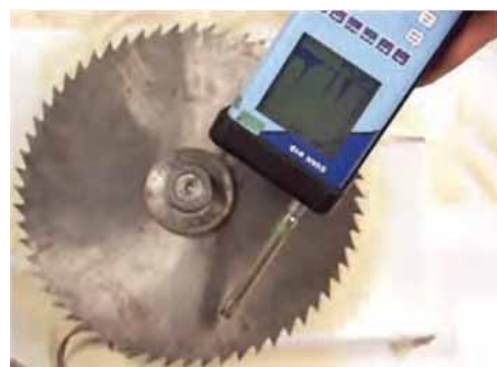
Fig. 5. FFT measurement with the Svan 912 meter
