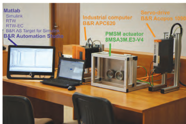
Fig. 5. Workstation for rapid prototyping control systems for the PMSM motor drives
