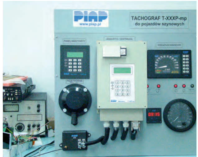
Rys. 9. Tachograf kolejowy T-130P-mp Fig. 9. Railroad Tachograph T-130P-mp
